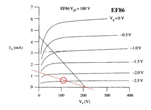
Databook pentode curves only for screen Vg2=150V. The AC load line is about 150k, due mainly to the 270k plate load, and 470k grid leak of the PI.
